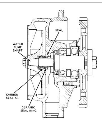
A small amount of coolant leakage across the surface of the "face-type" seals is normal, and required, to provide lubrication for this type of seal. A hole is provided in
